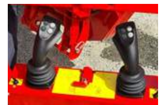
Optional electro-hydraulic controls with multifunctional levers
