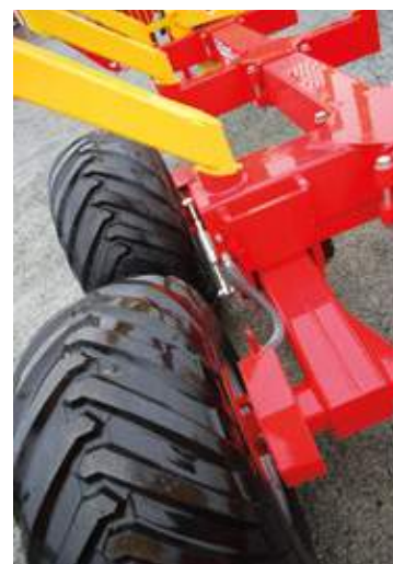
4 wheels hydraulically braked
