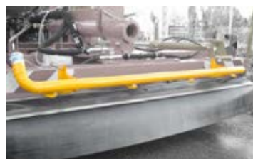
High pressure watering line, 4 sprayers
