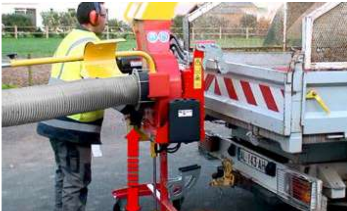
Hydraulic set-up at the rear of the truck, only 1 operator needed
