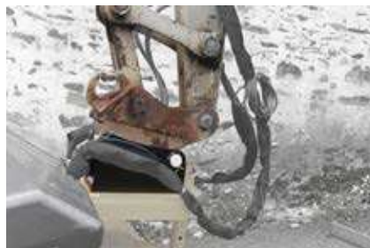
Quick fit coupling for excavator. Adaptation on all type of carrier and any coupling.
