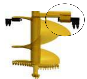
Auger with widening system
