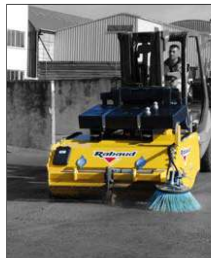
TURBONET 1500 AUTONOME + options : watering & side brush
