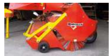
Collecting box, mechanical emptying
