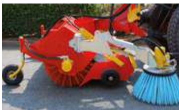
Side brush Ø 550 mm hoses, 3-way valve (standard version with central brush)
