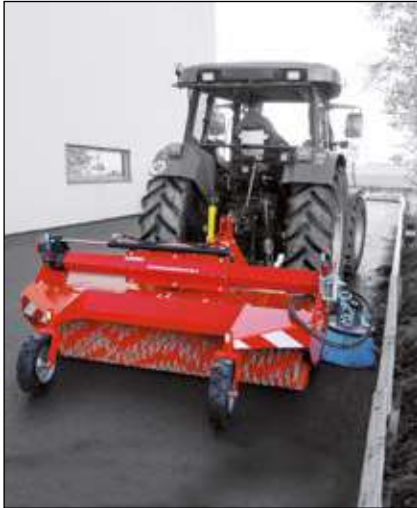
SUPERCHAMPION 2100 A with hydraulic offset & orientation+ side brush
