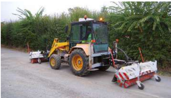
SETRACLEAN - Mounting on backhoe loader with rear SETRA plate + one mounted on the front loader
