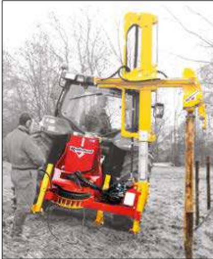
VIBRESCOPIC PRO with hydraulic extraction of the pre-hole bar
