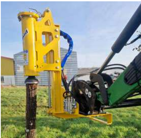
Pre-hole bar alone Ø 55 mm 1,30 m long
