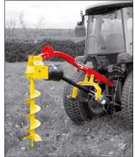
Hole digger MICROTRACTOR at work
