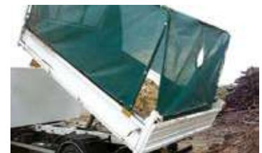
Casing kit door opening for unloading
