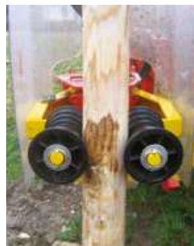
Post Driver TURBOFRAP 200 Hydraulic post-clamp with guiding rollers
