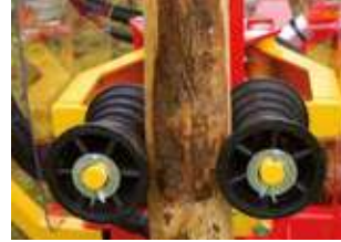
post clamp with guiding rollers
