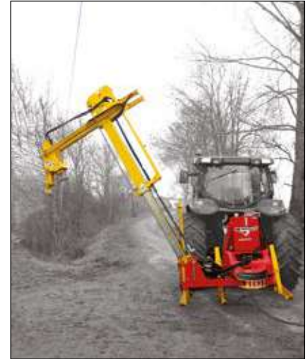
VIBRESCOPIC PRO, hydraulic tilt 18° inside / 25° outside
