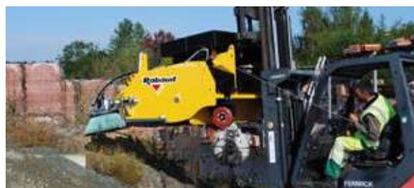
Collecting box emptying from the driver station
