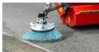
Side brush Ø 700 mm with rotation reverser
