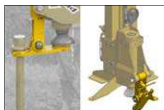
Pre-hole bar with hydraulic extraction
