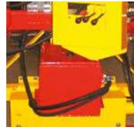
Hydraulic unit PTO 540 rpm 15 L/min. pump
