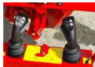
3 Electro-hydraulic controls by multifunctional levers
