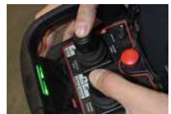
4 Electro-hydraulic controls by remote control
