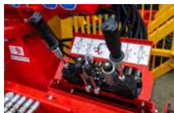
2 Hydraulic control with levers and electric control with buttons for the telescope and grapple
