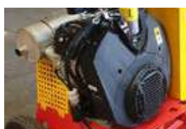
Heat engine POWER PACK 29,4 kW / 40 HP
