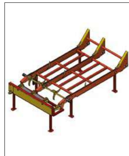
Loading deck with chains
