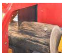
Saw blade with carbide teeth Cutting length adjustable by stop
