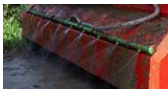
Watering by pressure, electrical pump 12V, 2 tanks of 150L, with spray line*
