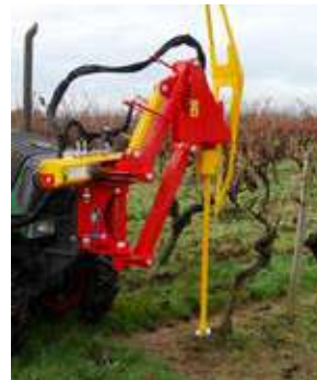
Hydraulic hole digger with mooring
