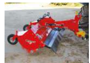
SUPERCHAMPION 2400 A with hydraulic orientation and offset with cylinder
