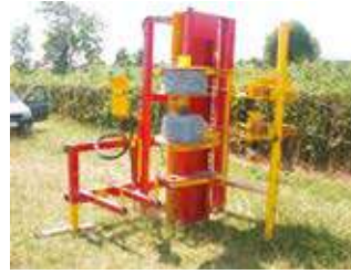
CLOTURMATIC GRX with 2 rows barbed wire uncoiler
