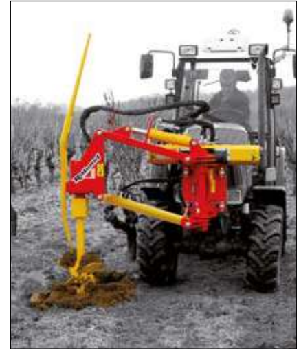
Hydraulic hole digger on vineyard tractor
