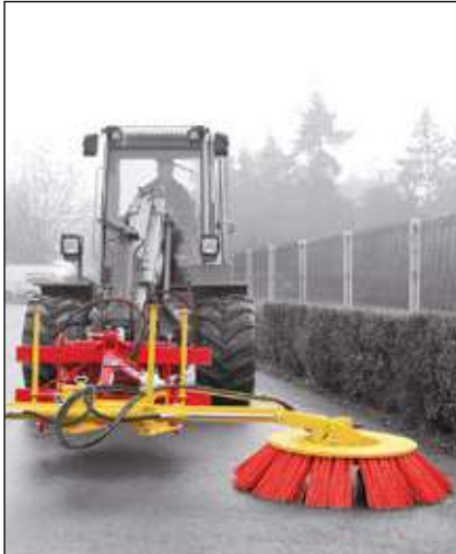
LOGENET with polypropylene brush
