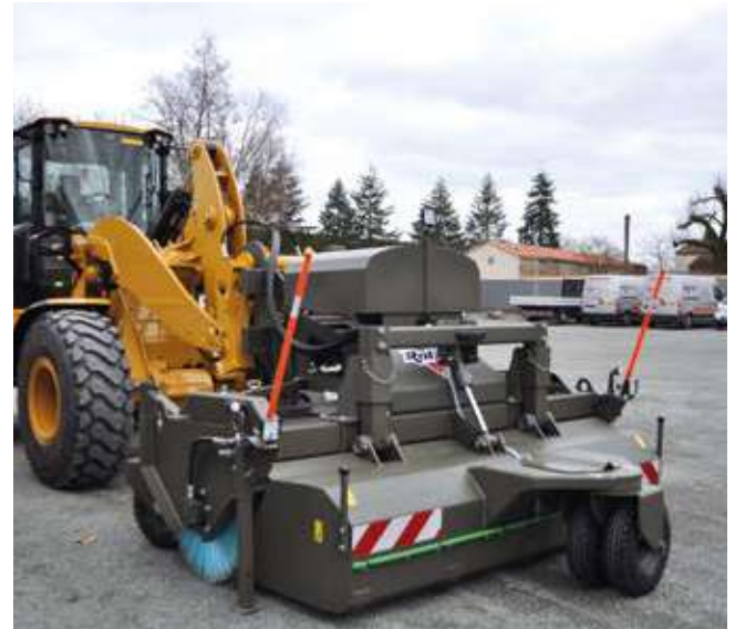
MEGANET 3000 with collecting box, watering system and specific painting
