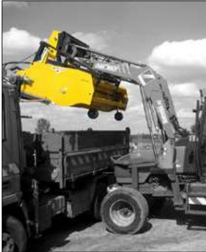
Emptying of the TURBONET mounting on loader
