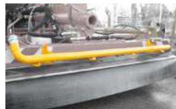
High pressure watering line, 4 sprayers
