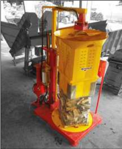
XYLOPACK with screener and buffering storer
