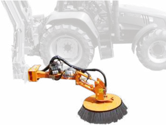
HERBIONET BE with brush Ø 750 mm
