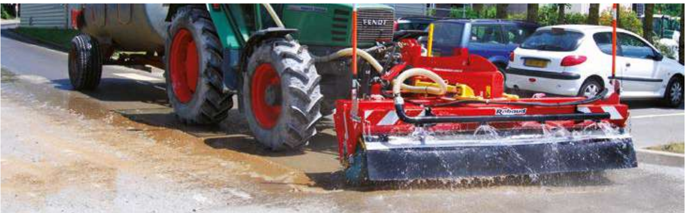
PROCHAMPION on tractor front 3-point linkage
