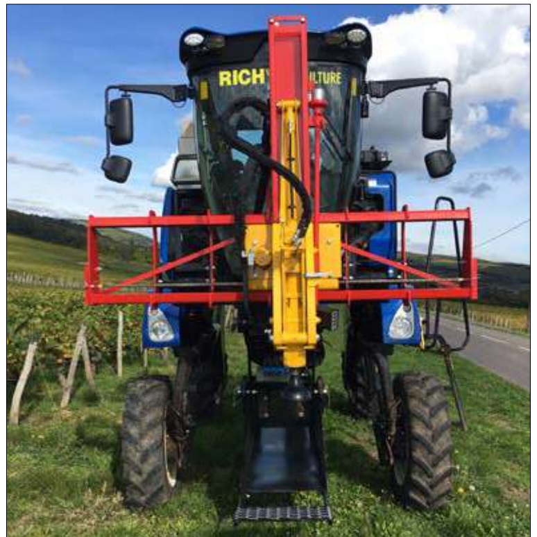
Special assembly : VIBRESCOPIC II STILTOR side shift of 0,75m right – left
