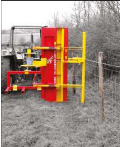
CLOTURMATIC GRX 4020 + 1 row barbed wire unwinder
