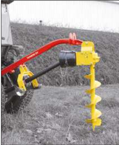
Hole digger MICROTRACTOR at work
