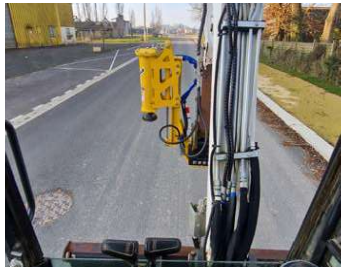
6-way hydraulic valve + control box in cabin + winding electric cord 15m or lead extension 12m
