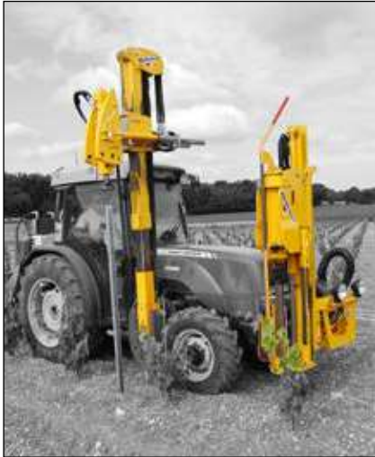
VIBRESCOPIC II BETWEEN WHEELS + Pre hole bar driver
