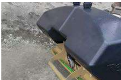
Option pressure watering. 2 water tanks of 150L. 12V or 24V electrical socket.
