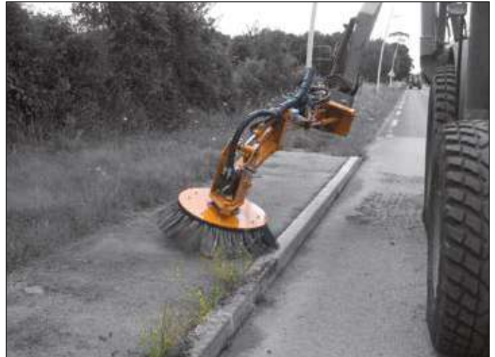
HERBIONET BE with brush Ø 750 mm
