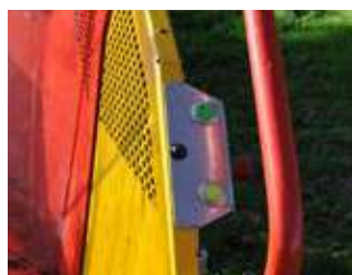
Push buttons : forward direction, reverse direction and STOP
